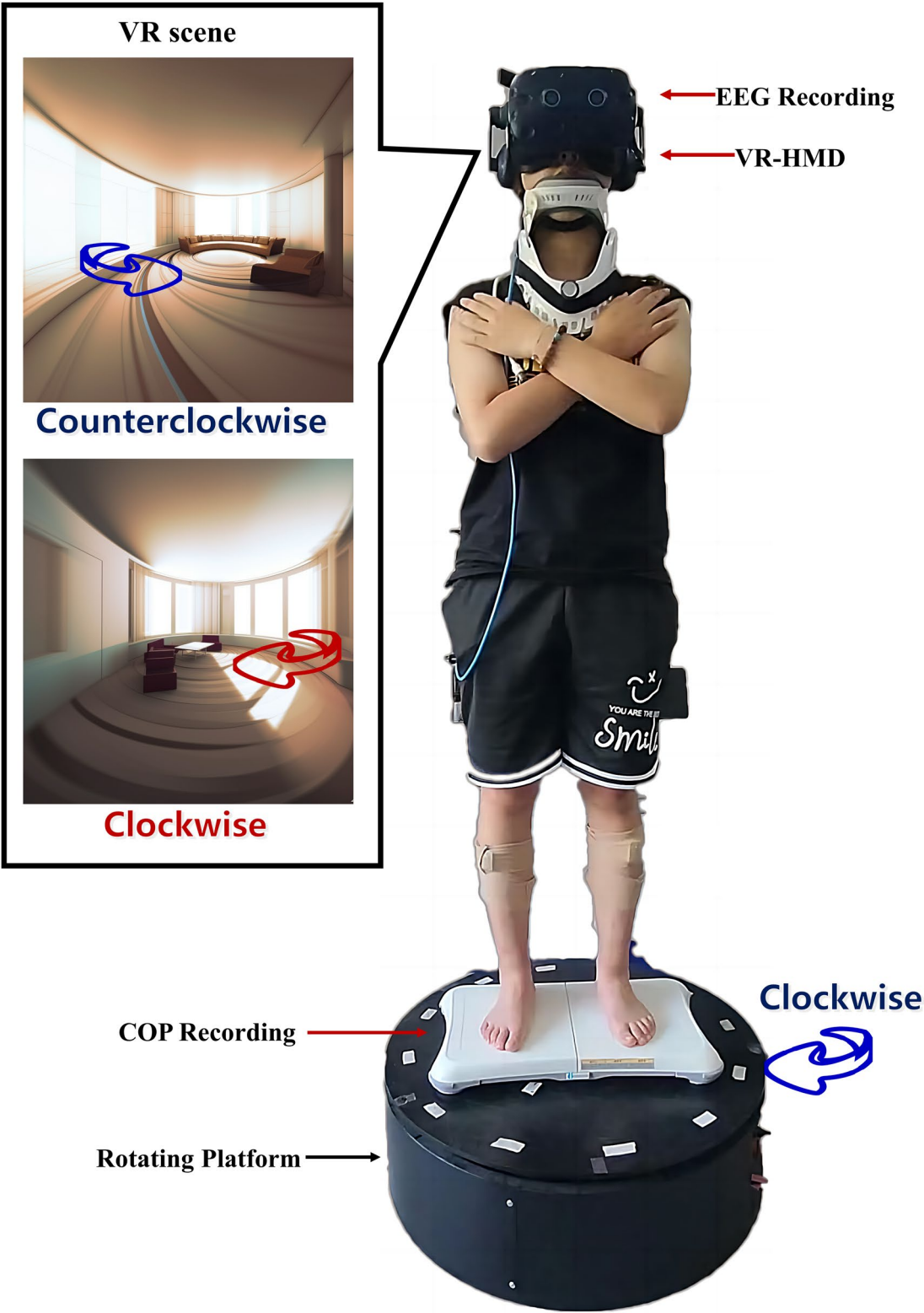
Fig. 1 Schematic diagram of the experimental setup and installation. The schematic diagram illustrates the experimental setup used to study the impact of Tai Chi on postural control under sensory perturbation conditions. Participants stood barefoot on a Wii Balance Board placed in the center of a rotating platform, with a virtual reality (VR) headset providing visual stimuli. Two conditions were tested: “sensory congruent” and “sensory conflict.” In the sensory congruent condition, visual and actual rotational movements were aligned, whereas in the sensory conflict condition, the visual scene was counter-rotated to create a mismatch between visual and proprioceptive inputs. Electroencephalographic (EEG) data were recorded using a 64-channel EEG cap, and center of pressure (COP) data were collected to assess postural stability
