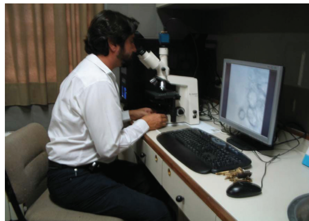
Figure 1. Zeiss microscope mounted on an antivibration table (Wentworth Laboratories, Ltd., Sandy, Bedfordshire, U.K.). Specimens are examined using a \times 100 interference contrast lens. Beating ciliated edges were recorded using a digital high-speed video camera (Prosilica Cam recorder; Allied Vision Technology) at a rate of 400 frames/s, using a shutter speed of 1 in 4000.
