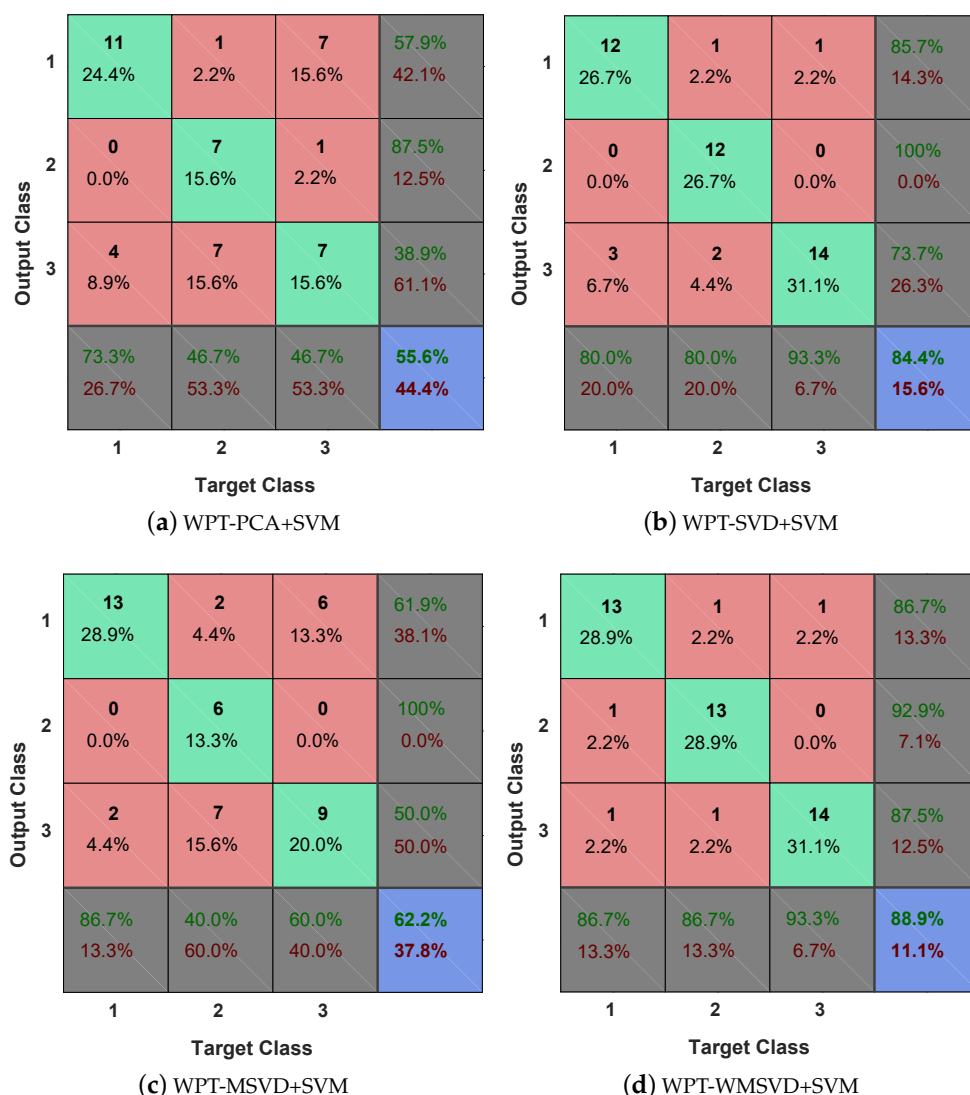
Figure 8. Classification confusion matrix of four algorithms: (a) WPT-PCA+SVM; (b) WPT-SVD+SVM; (c) WPT-MSVD+SVM; and, (d) WPT-WMSVD+SVM.
