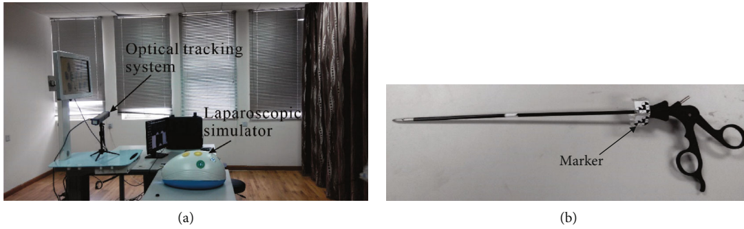
FIGURE 1: Experimental platform: (a) laparoscopic simulator and optical tracking system and (b) laparoscopic instrument with markers.
