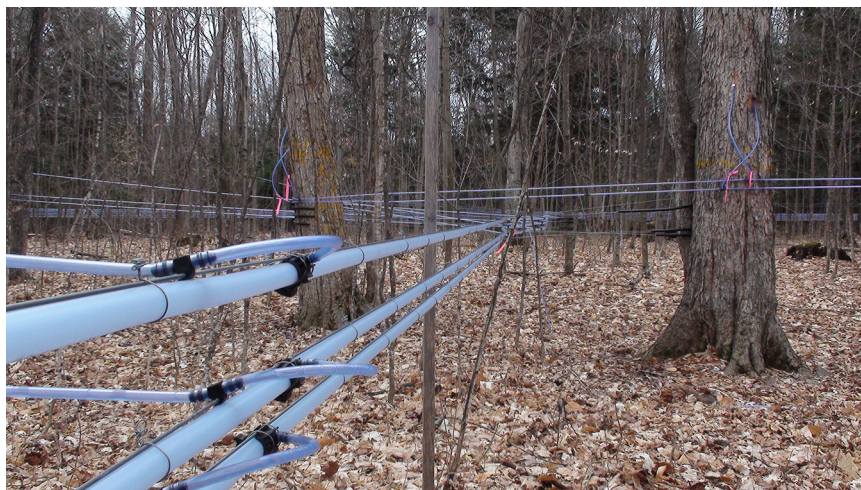
Fig. 1. Example of plastic tubing system used to collect maple sap showing lateral and main lines and spouts connected to trees.
