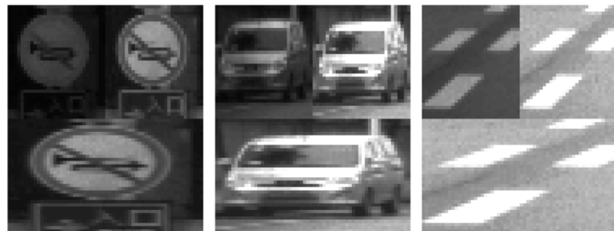
Figure 6. Three sample parts of source RCCC image decomposed into three images: two small images with R and C1 components and a horizontally two times larger image comprising C2 and C3 components.
