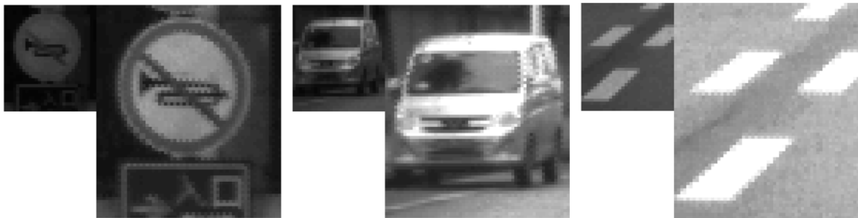
Figure 4. Three sample parts of source RCCC image decomposed into two images with R and CCCC components (the second image is created with the CCC components while the missing values are interpolated).
