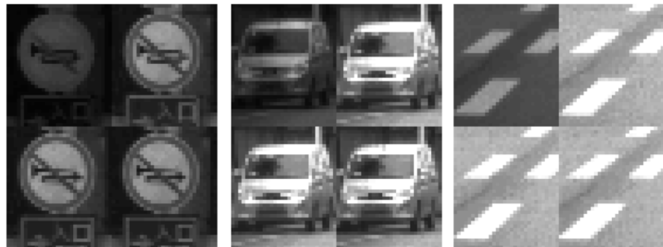
Figure 5. Three sample parts of source RCCC image decomposed into four images with all components R, C1, C2, C3 separated.
