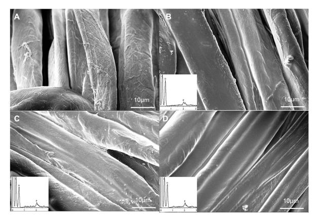
**Figure 6.** SEM micrographs of COT (**A**), COT\_DNA 5% (**B**), COT\_DNA 10% (**C**) and COT\_DNA 19% (**D**) at 5000× and elemental analyses Reproduced with permission from [44]. Copyright 2013, Elsevier.
