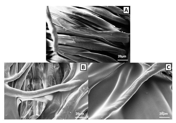
**Figure 4.** SEM magnifications of untreated cotton (**A**), cotton treated with caseins (**B**) and cotton treated with hydrophobins (**C**). Reproduced with permission from [38]. Copyright 2014, Elsevier.
