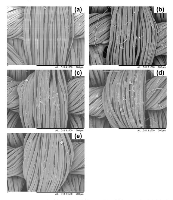
**Figure 9.** SEM micrographs of the untreated silk fabric (**a**) and the silk fabrics treated with the hybrid sols unmodified (**b**) and modified by APDTMS (**c**), CPTS (**d**) and MPTS (**e**). Reproduced with permission from [57]. Copyright 2018, Elsevier.
