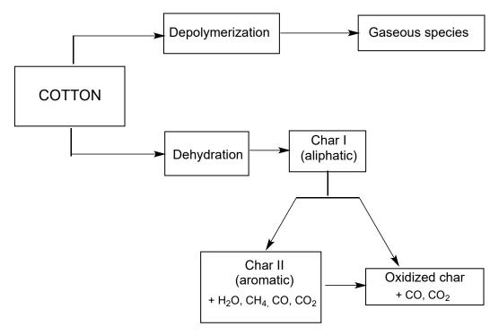
Figure 2. Scheme of cotton degradation.
