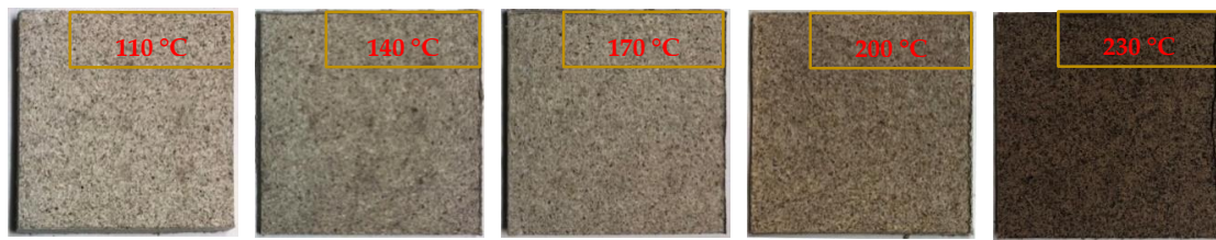
Figure 2. Bio-board produced at different heating temperature.
