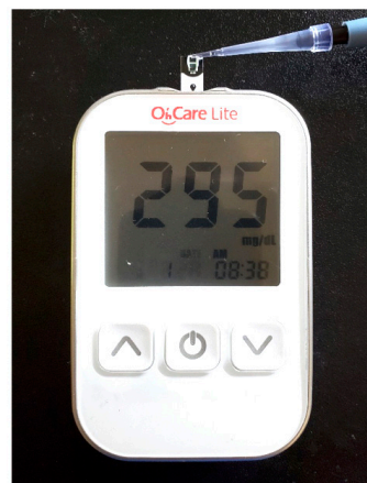
FIGURE 2. P10 micropipette used to load glucose solution into test strip. The glucose meter provides a measurement of glucose concentration in milligrams per deciliter after a short countdown.
