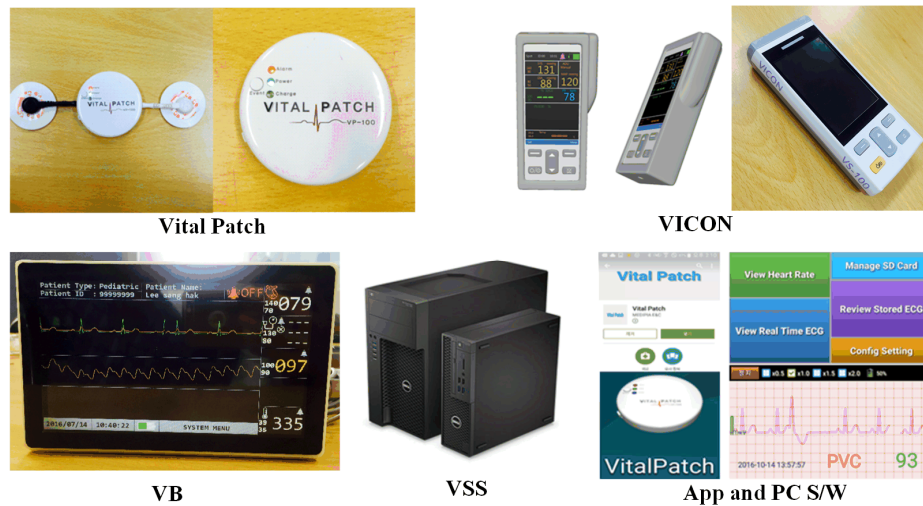
Figure 11. Developed vital sign measurement devices (Vital Patch (VP), VICON), VB, VSS, and App, and PC S/W).
