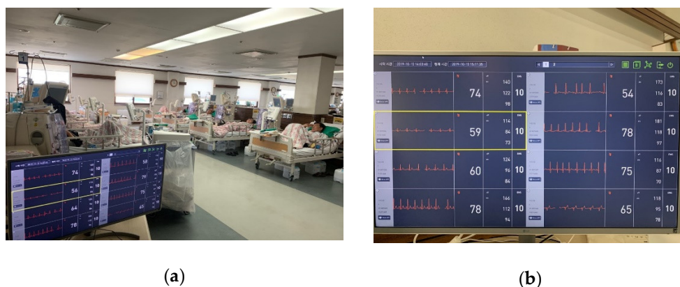
Figure 19. Proposed u-Vital system applied for a real hospital; (a) artificial kidney room and (b) central monitoring in VSS.
