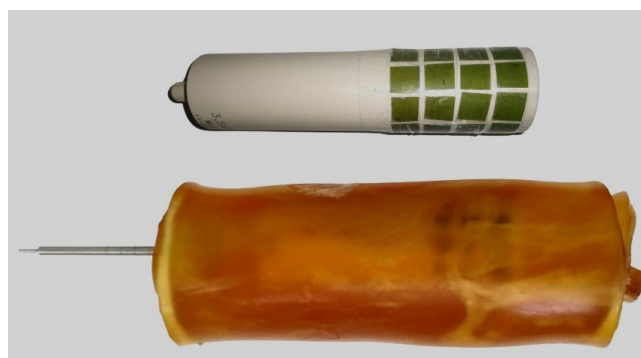
Fig. 3. (Top) Applicator surface taped with EBT3 Gafchromic films. (Bottom) Tandem and vaginal cylinder assembly wrapped in elasto-gel bolus.
