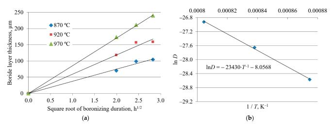
**Figure 5.** Growth kinetics of boride layers on C15 steel: (**a**) Boride layer thickness as a function of the square root of the boronizing duration; (**b**) natural logarithm of growth rate constant as a function of the reciprocal boronizing temperature [43]. Reprinted with permission from ref. [43]. Copyright 2012 Mechanical Engineering Faculty in Slavonski Brod.
