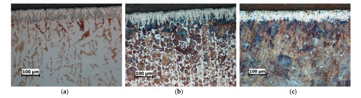
**Figure 2.** Microstructure of the boride layers obtained by boronizing at 870 °C for 4 h, magnification 200:1: (a) C15 steel; (b) C45 steel; (c) C70W2 steel.
