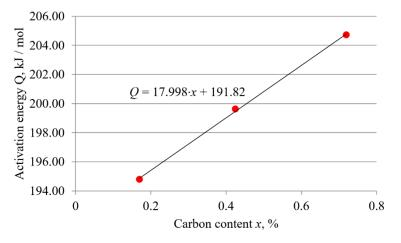
Figure 9. Relationship between the activation energy and the carbon content of steel.
