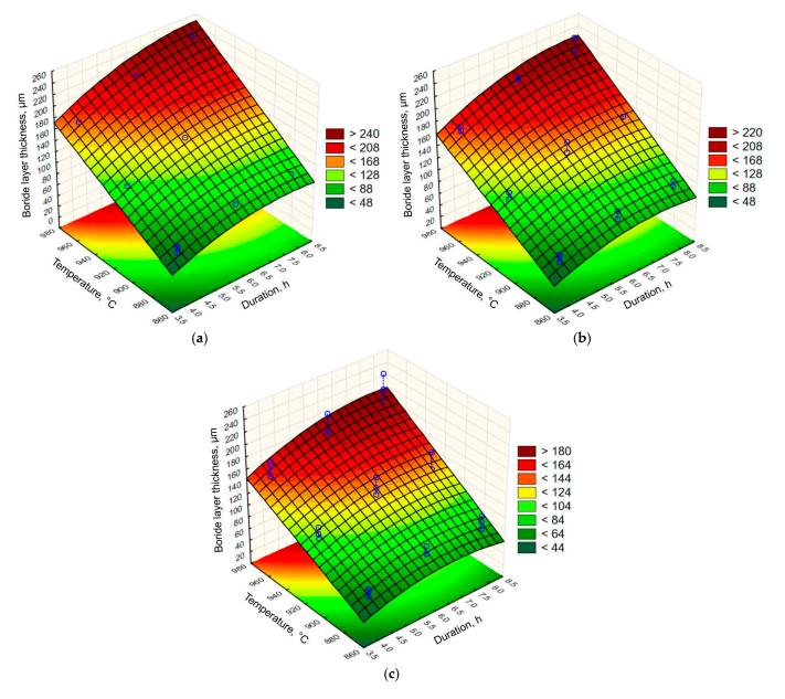
**Figure 10.** Relation between the boride layer thickness and the boronizing temperature and duration for: (**a**) C15 steel; (**b**) C45 steel; (**c**) C70W2 steel.
