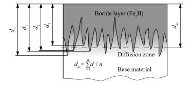
**Figure 1.** Determination of the boride layer thickness [43]. Reprinted with permission from ref. [43]. Copyright 2012 Mechanical Engineering Faculty in Slavonski Brod.
