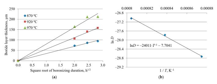
**Figure 6.** Growth kinetics of boride layers on C45 steel: (**a**) Boride layer thickness as a function of the square root of the boronizing duration; (**b**) natural logarithm of the growth rate constant as a function of the reciprocal boronizing temperature [44]. Reprinted with permission from ref. [44]. Copyright 2016 Croatian Metallurgical Society.
