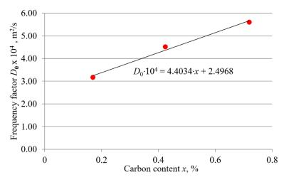
Figure 8. Relationship between the frequency factor and the carbon content of steel.
