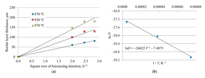
**Figure 7.** Growth kinetics of boride layers on C70W2 steel: (a) Boride layer thickness as a function of the square root of the boronizing duration; (b) natural logarithm of growth rate constant as a function of the reciprocal boronizing temperature [43]. Reprinted with permission from ref. [43]. Copyright 2012 Mechanical Engineering Faculty in Slavonski Brod.
