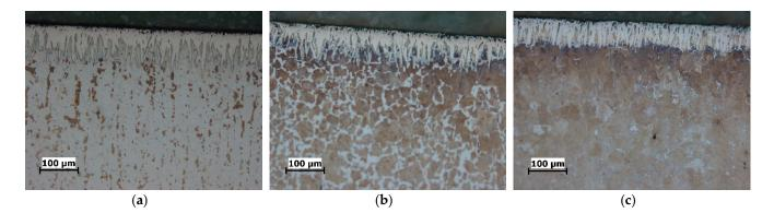
**Figure 3.** Microstructure of the boride layers obtained by boronizing at 870 °C for 8 h, magnification 200:1: (a) C15 steel; (b) C45 steel; (c) C70W2 steel.
