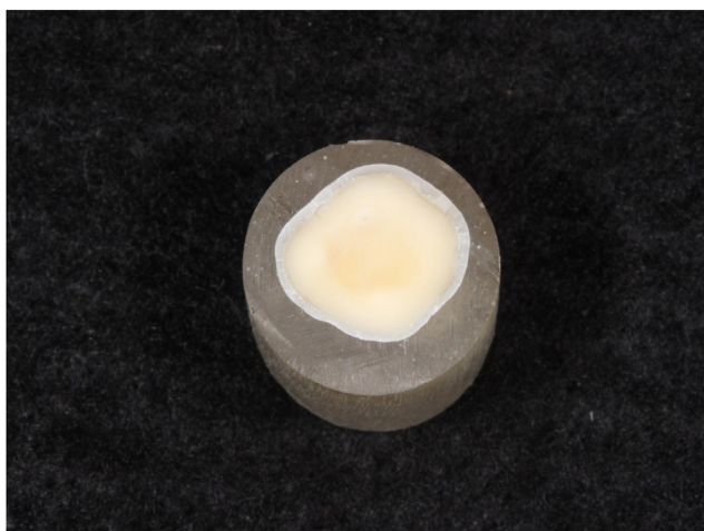
Figure 1 Cross-sectional surface of the teeth was ground flat with water-cooled stone trimmer followed by polishing with 240-grit and 600-grit abrasive sandpapers.
