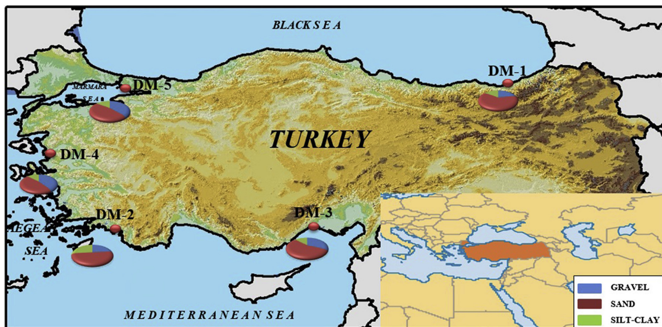
Fig. 1. Five sampling points in the shores of Turkey and their pie charts showing the particle size distributions (Source: TUBITAK MAM Environment and Cleaner Production Institute Geographic Information System Group).
