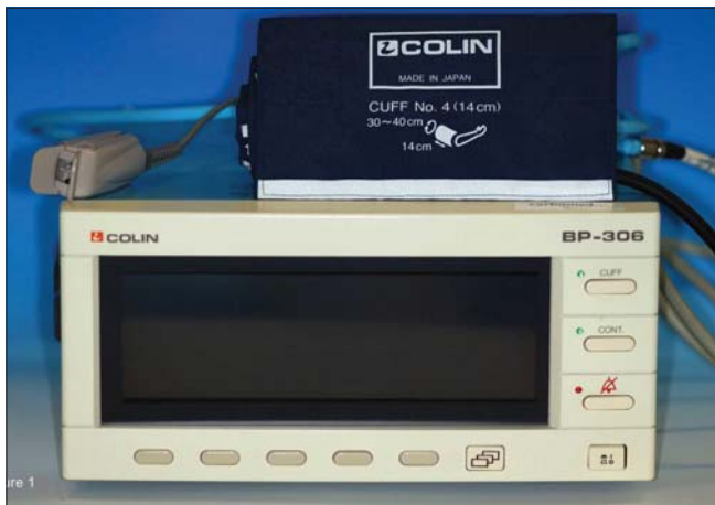
Figure 1: Colin BP 306 compact monitor (Colin Corporation, Japan) with blood pressure cuff and finger clip
