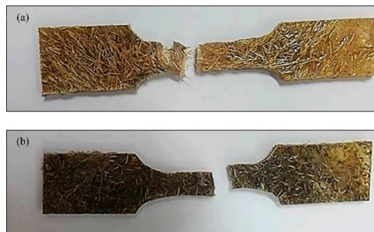
Figure 6. Specimens after tensile testing: (a) r-EPS/5% t-coir, and (b) r-EPS/5% t-BSF.
