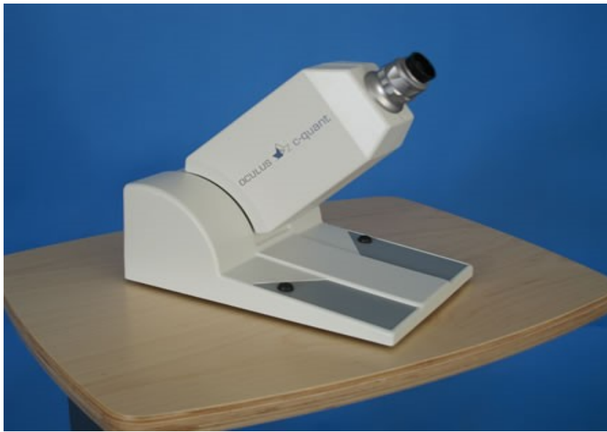
Figure 1. C-Quant equipment. Left and right black buttons located on the silver area at the base were used to the 2-Alternated Forced Choice left–right judgment.
