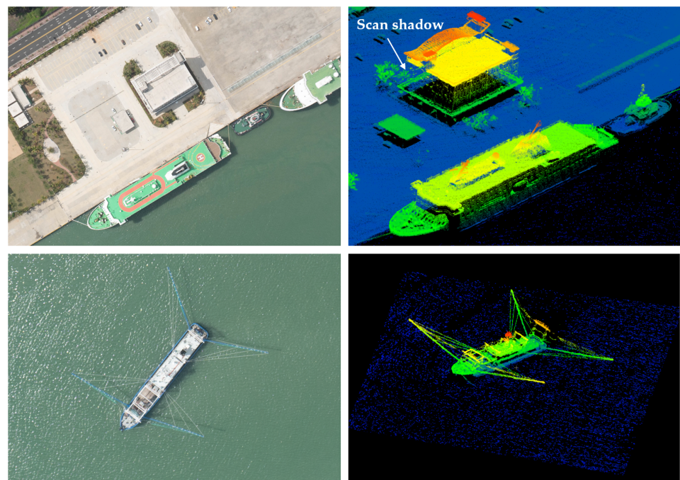
Figure 14. Left: The aerial picture of the passenger ship and trawl boat docked at Wenchang City and offshore ocean area, respectively. Right: The lidar image of the ships was acquired by a single pass at the altitude of 0.5 km and the mean point density is 598.8 pts/m 2 . The point cloud is colored according to its elevation. The dark blue in the lidar image is the ocean surface.
