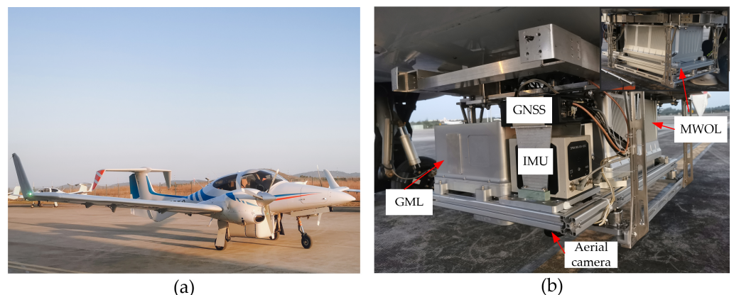
Figure 5. (a) The Diamond DA-42MPP aircraft on the tarmac at Wuhu Xuanzhou Airport; (b) photograph of the airborne multispectral lidar system mounted on the aero belly. A back view of the system is displayed in the inset.
