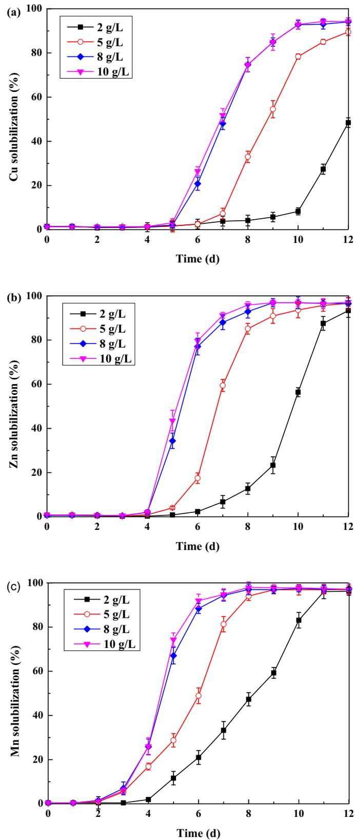
**Fig. 4.** The metal solubilization at different sulfur concentrations (a) Cu, (b) Zn, (c) Mn during the bio-leaching process.
