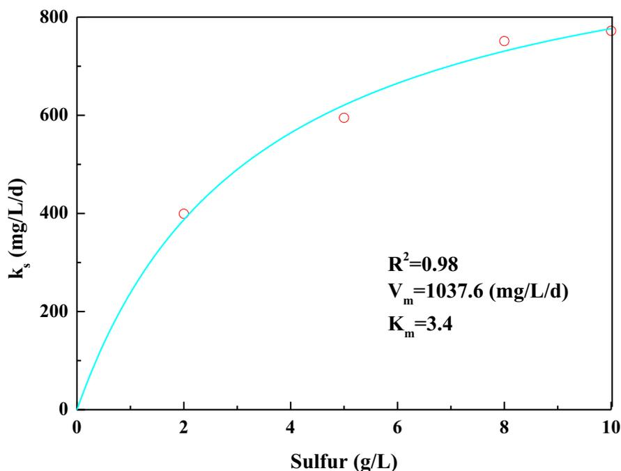
**Fig. 3.** Sulfate production rate at different sulfur concentrations during pig manure bioleaching process (the solid line represents the fit to Michaelis-Menten type of equation).
