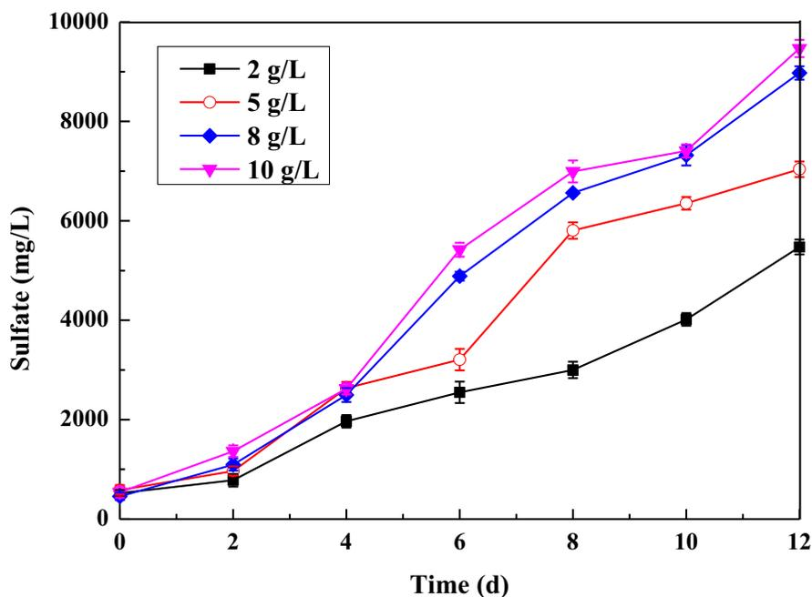
**Fig. 2.** The variations of sulfate in bioleaching process for different sulfur concentrations.
