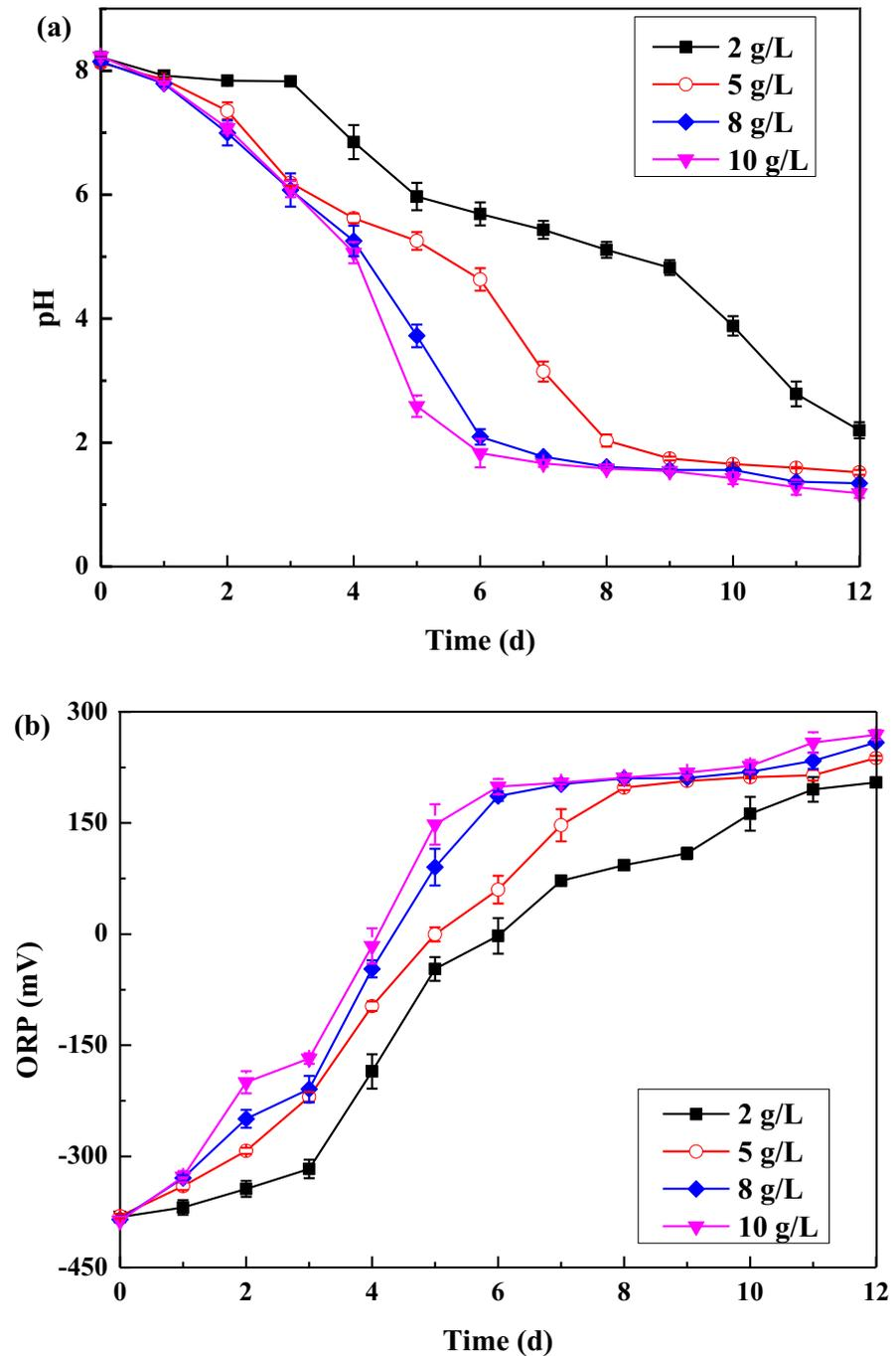
Fig. 1. Changes of pH (a) and ORP (b) in bioleaching process for different sulfur concentration.
