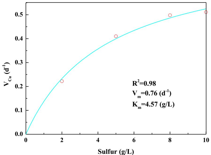
**Fig. 5.** Relationship between rate of Cu solubilization and sulfur concentration (the solid line represents the fit to Michealis–Menton type of equation).
