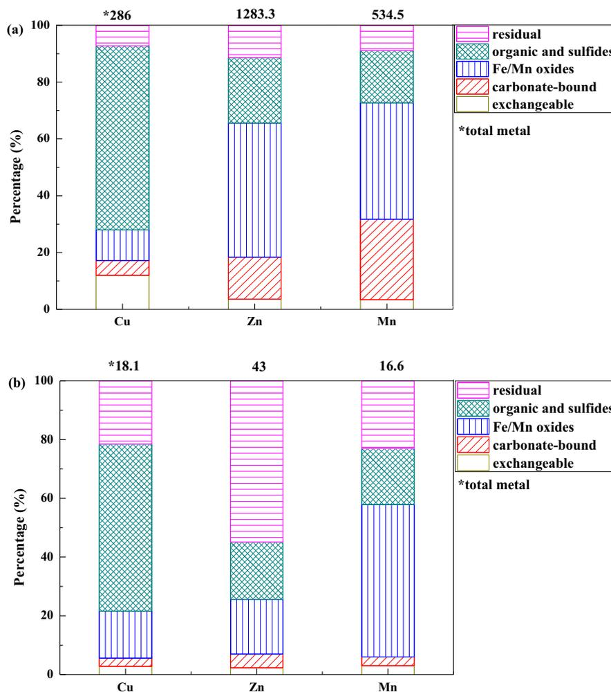
**Fig. 6.** Metal speciation in pig manure before (a) and after (b) the bioleaching process.
