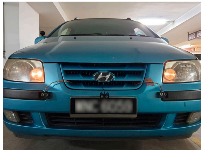
Figure 3. Installation of ultrasonic sensors and Garmin lidar on the vehicle.
