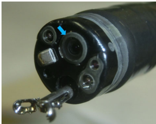
Figure 3. A picture of the tip of the endoscope. The blue arrow indicates the objective lens located at the upper side.
