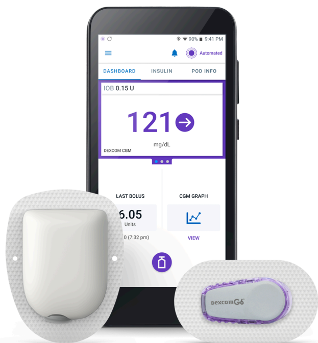
FIGURE 1 Components of the Omnipod 5 AID system: (left) the tubeless Pod containing the AID algorithm; (center) the app, pictured running on a smartphone; and (right) the Dexcom G6 inter-operable CGM sensor. The Pod is a lightweight, waterproof (IP28), self-adhesive insulin pump that delivers insulin via an automatically inserted cannula. The algorithm receives glucose measurements every 5 minutes from the on-body CGM sensor and engages the Pod to deliver microboluses every 5 minutes based on current and projected glucose levels, aiming for a set target glucose value in its calculations. Users interact with the system through the app, which communicates wirelessly with the Pod. Actions performed via the app include completing initial setup and programming pump settings, activating and deactivating Pods, starting automated mode, using the bolus calculator/delivering boluses, enabling the Activity feature, viewing insulin delivery and CGM history, responding to system alerts and alarms, checking Pod status, and adjusting pump parameters. The app home screen displays the current CGM value and trend, the amount of IOB, information about the most recent bolus, and a link to view a CGM history graph. The bolus calculator is accessed using the circular icon near the bottom of the screen. Because the algorithm runs on the Pod and the Pod and CGM are both worn on-body and communicate directly, AID can continue uninterrupted even if the handheld device containing the app is not nearby. Image used with permission. ©2020 Insulet Corp.
