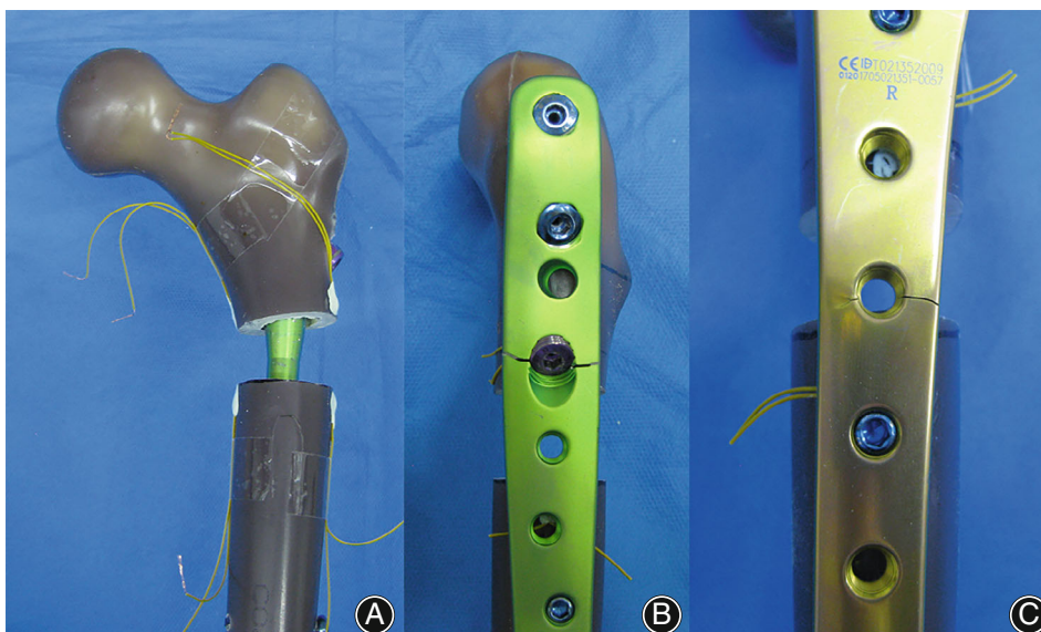
Fig. 6 Failure modes of the implants. (A): Failure mode of PFNA in the axial compression failure testing. The main nail of the PFNA was curved at the proximal part; (B): Failure mode of PFLP in fatigue testing. PFLP constructs a fracture at the level of the fourth screw hole of the plate; (C): Failure mode of LISS in fatigue testing. A fatigue crack emerged at the hole at the fracture site
