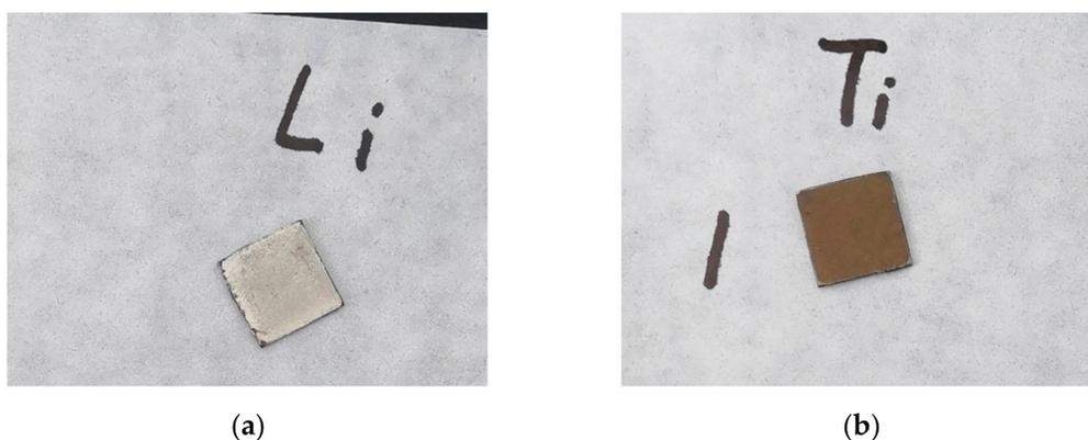
**Figure 2.** Photograph of sample (1) and sample (2): (a) sample (1) after being exposed to the air for a minute; (b) sample (2) after being exposed to the air for a minute.
