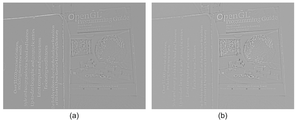
Figure 4. High frequency of input images: (a) High frequency of near focused image, (b) High frequency of far focused image.
