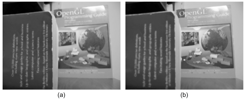
Figure 3. Low frequency of input images using the EAC: (a) Low frequency of near focused image, (b) Low frequency of far focused image. It is evident that the EAC preserves the strong image edges.
