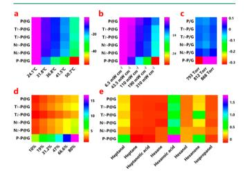
Figure 3. Heat maps represent the responses of BLSA to temperature (a), light exposure (b), air pressure (c), relative humidity (d), and volatile organic compounds (e).
