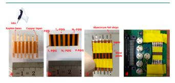
Figure 2. (a-c) Images giving examples of the design and fabrication of a 6-lane BLSA by different inks integrated on a Kapton film. (d) BLSA fixed onto an electronic board for testing.
