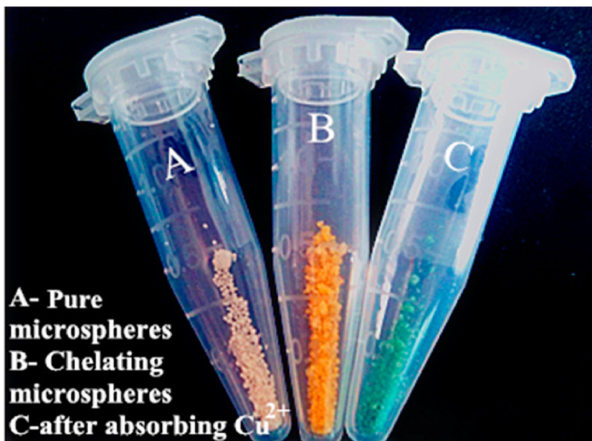
Figure 7. Typical photographs of pure PVMA microspheres, chelating microspheres, and the microspheres after adsorbing \text{Cu}^{2+} (Reproduced with permission from Zhang et al. [48], Copyright 2016, American Chemical Society).
