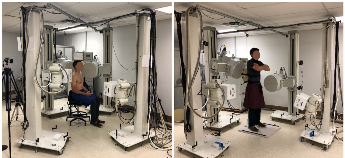
Fig 2. Biplane radiography setup. (Left) Cervical spine setup with two offset systems and interbeam angle of 55°, 16" image intensifiers and high-speed cameras. One system is oriented parallel to the horizontal and the other is oriented above the horizontal. (Right) Lumbar spine setup with attached attenuator and orthogonal systems. One system is oriented parallel to the horizontal and the other is oriented above the horizontal. Note: Validation was performed using a cadaveric specimen; however, the setup is demonstrated with a live subject. Lumbar acquisition was performed with the cadaveric specimen inverted and the AP system oriented 8° above the horizontal.
