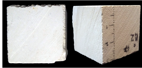
Figure A1. Example of the Ançã stone samples used for this study.
