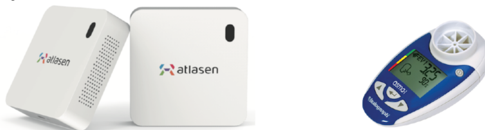
Figure 4. Images of an indoor air quality sensor that measures PM 2.5, CO 2 , and NO 2 (left) and a spirometer that measures FEV1, FEV6, and % of personal best FEV1 (right).
