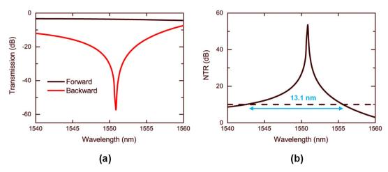
Figure 4 | (a) The forward and the backward transmission spectra, with incident power  $P = 390 \mu W$ . (b) The NTR spectrum.
