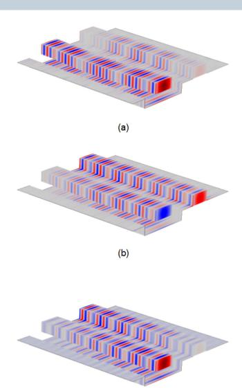
Figure 6 | Y component of electric field along the waveguide. (a) Light is launched into Port 1,  $P=390~\mu W$ . (b) Light is launched into Port 4,  $P=390~\mu W$ . (c) Light is incident from Port 1 and outputs from Port 4,  $P=1~\mu W$ .
