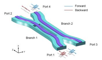
Figure 1 | Schematic illustration of the asymmetric optomechanical coupler. Branch 1 is a freestanding silicon waveguide in close proximity to the underlying silicon dioxide substrate. Branch 2 is a conventional stripe waveguide fixed on the substrate. The backward transmission light is incident from Port 1, and emits from Port 4. The forward transmission route is just opposite.
