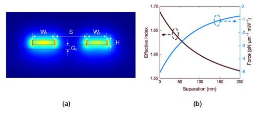
Figure 2  $\mid$  (a) Mode profile of the cross section. (b) Effective index and optical gradient force of Branch 1 versus the separation d between Branch 1 and the substrate.
