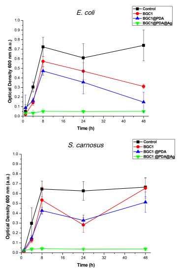
**Figure 6.** Turbidity measurements on suspensions of both tested *Staphylococcus carnosus* and *Escherichia coli* strains in lysogeny broth (LB) medium on different samples, showing their different antibacterial effects.
