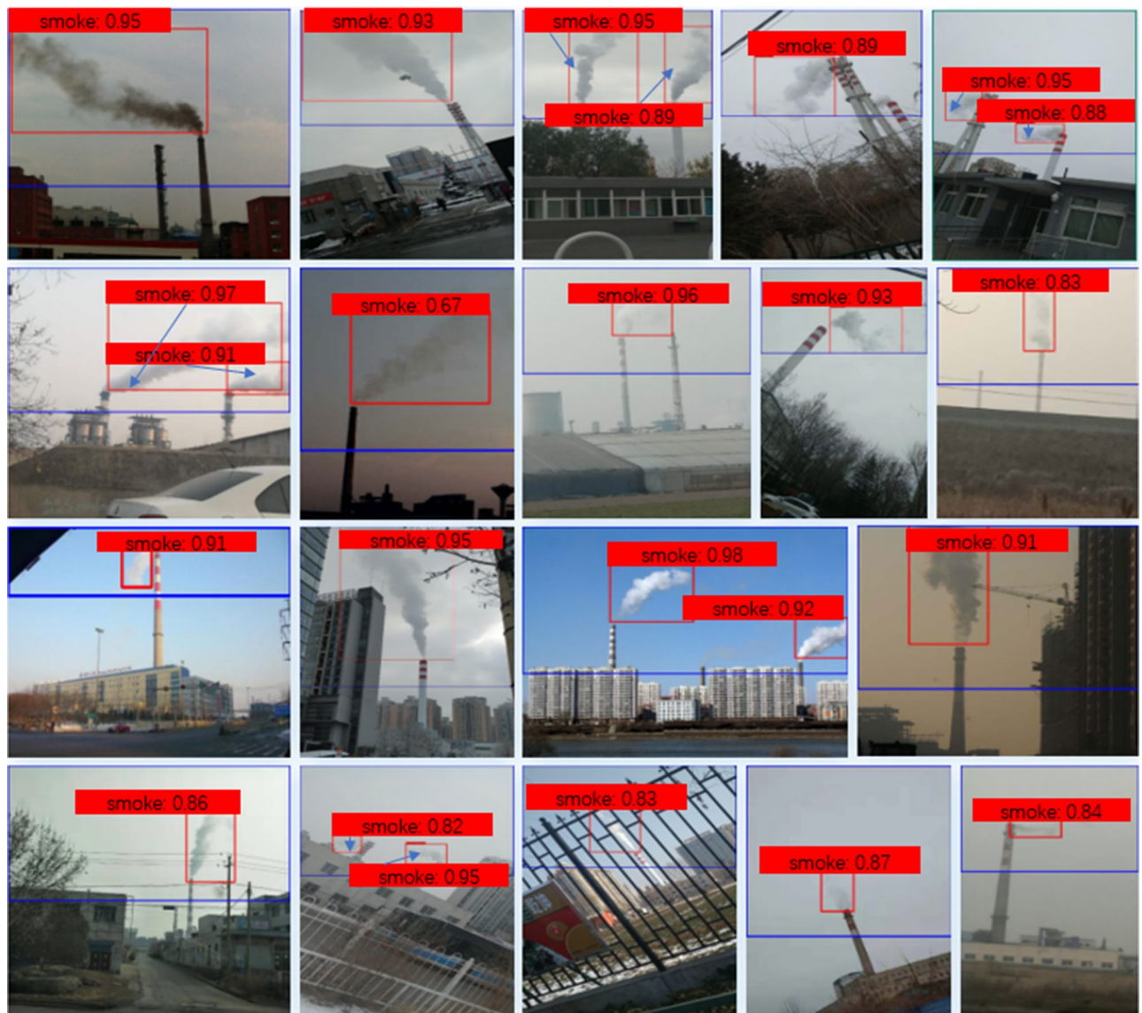
Figure 11. Visual effect of TSSD algorithm on detecting factory smoke. Four-class smoke images of dataset are all included. Blue boxes represent the reduced detection range, and red boxes show the detected smoke region. The text on top of each bounding box represents the confidence of smoke detection.
