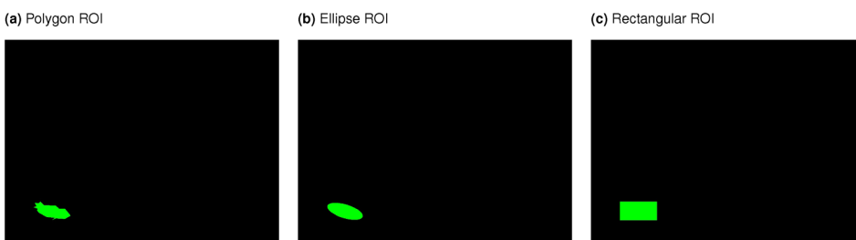
Figure 2. Automatically detected ROIs, which were based on taking the difference between the original and changed image, thresholding, detecting bounding areas (polygons), fitting either bounding polygons, ellipses or rectangles around these areas with a minimum surface area (to avoid fitting regions around noise). The procedure differs from that reported in a poster in that bounding boxes were fitted around detected polygons, rather than on the thresholded image, avoiding fitting boxes are noise pixels.
