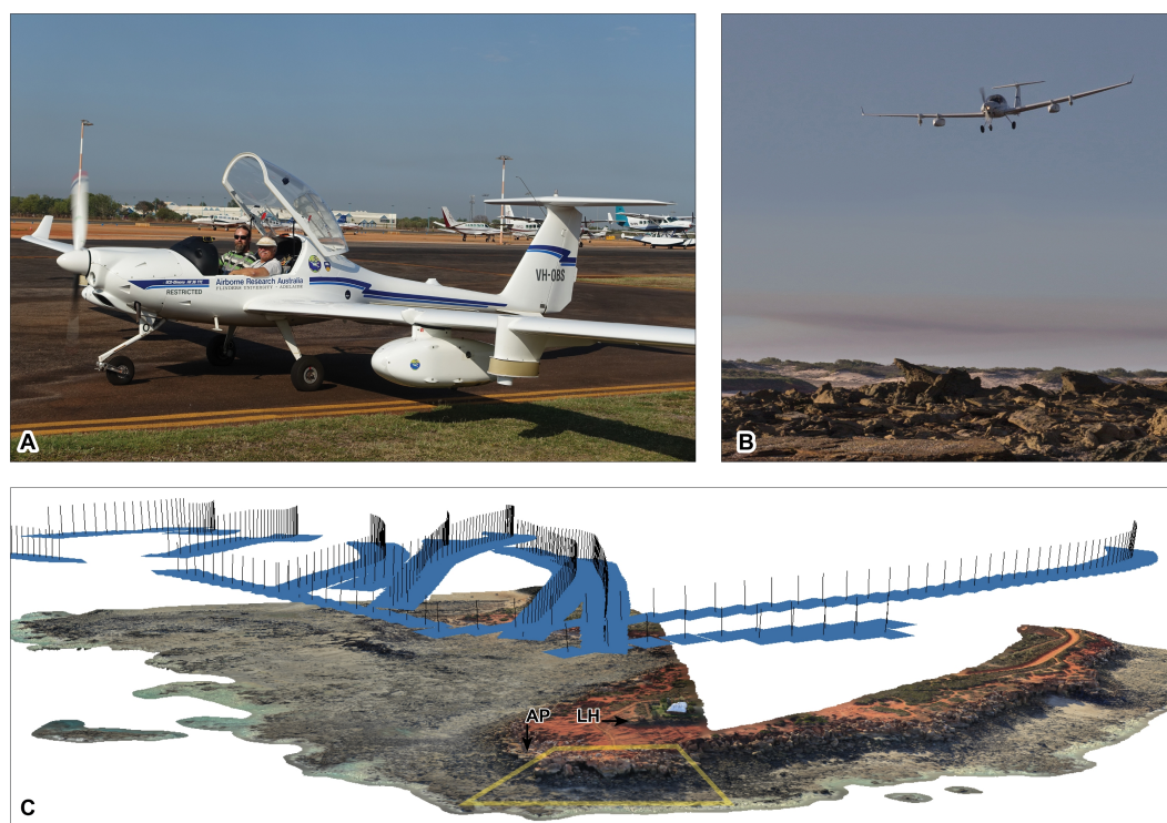
Figure 6 Photographic and laser data acquisition methods used from manned aircraft on Broome Sandstone dinosaurian tracksites. (A) Diamond Aircraft ECO-Dimona with SWS and JH (pilot). (B) ECO-Dimona over tracksite undertaking laser scanning and photography. (C) point cloud of the intertidal zone at Minyirr, derived from photographs. The blue rectangles indicate spatial position of the camera and the path taken by the aircraft. The yellow outline indicates the portion of Minyirr (UQL-DP56) that was the focus of the current study (2.4 ha). Note that laser scanning occurred simultaneously and continuously during photographic data acquisition. Total area of C equals approximately 13 ha. Photograph credit (B): Damian Kelly.
