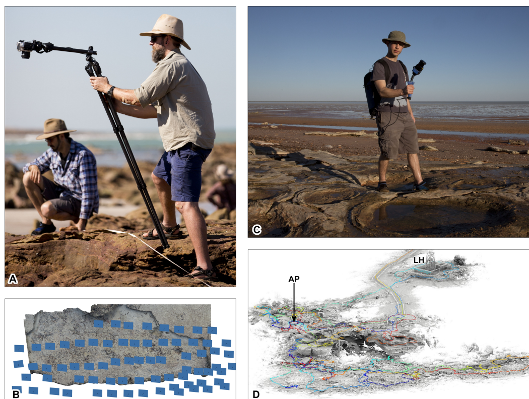
Figure 4 Ground-based data acquisition techniques used on Broome Sandstone dinosaurian tracksites. (A) Ground-based photography (left to right: AR and SWS). (B) photogrammetry-derived orthophotographic mosaic of the track-bearing platform UQL-DP56-4, -5 and -9 (blue rectangles indicate spatial position of the camera). (C) 'Zebedee' handheld ground-based laser scanning (RZ). (D) point cloud of Minyirr (UQL-DP56). Colored line indicates path taken whilst scanning. Area of B and C equals approximately 20 m 2 and 4 ha, respectively. Abbreviations: AP, Anastasia's pool; LH, Lighthouse. Photograph credit (A, C): Damian Kelly.
