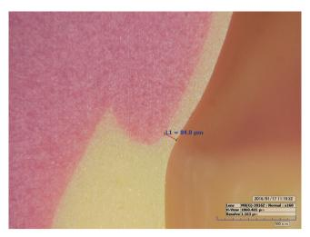
**Fig. 5.** Marginal gap measurement analysis using digital microscope (×160 magnification).
