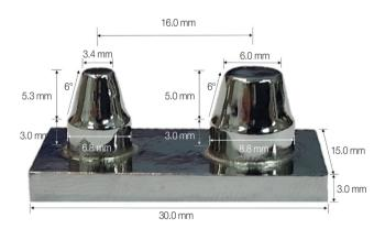
Fig. 2. Dimensions of three-unit master model in metal casting.
