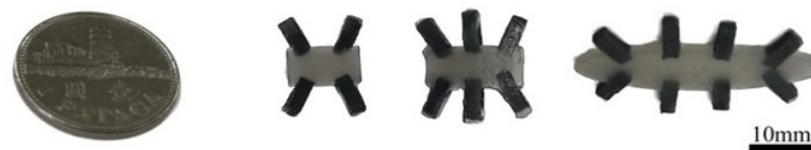
**Figure 2.** Prototype of quadrupedal, hexapodal, octopodal robots, and a 1-pataca coin.
