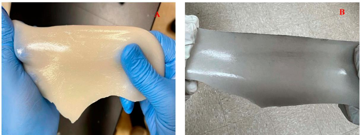
Figure 3. Picture of (A)  $\text{Si}_3\text{N}_4\text{MgHNT}$  and (B)  $\text{Si}_3\text{N}_4$  Hydrogel Patch.
