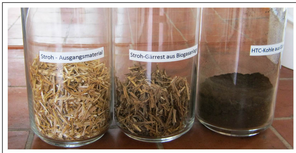
Figure 6. (Left to right) Dry wheat straw, dry wheat straw digestate, and HTC biochar of wheat straw digestate. This is the real time image of the different states of wheat straw. Here in this figure, the effect of anaerobic digestion (AD) and HTC can be visible. The fiber structure is still visible in the digestate, while it becomes powdery after HTC.
