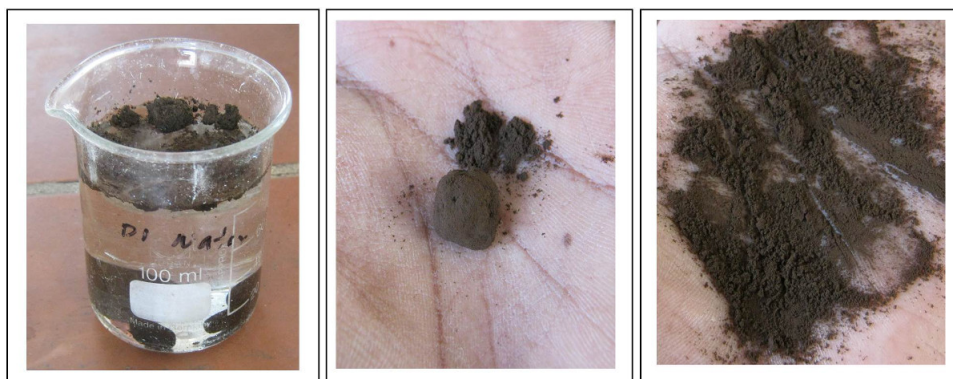
Figure 7. Hydrophobicity of the HTC biochar (left), friability of the HTC biochar (right). This is again the real time image of hydrophobicity and friability of HTC biochar. In the first image, HTC biochar is sunk under the water, while the next two images the condition of biochar before and after hard-crushing are shown.
