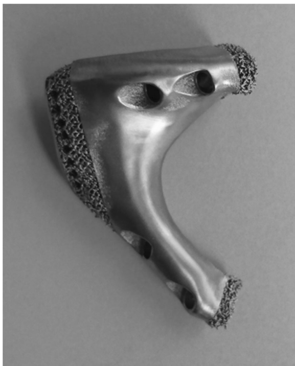
Fig. 4 Prosthesis fabricated with 70% porosity and 600- \mu m-pore size by electron beam melting technique
