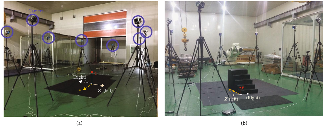
FIGURE 4: (a) Experimental environment for a camera setup (blue circles). (b) Position of the staircase. Yellow, red, and white arrows on the figures define the axes in coordinate space.
