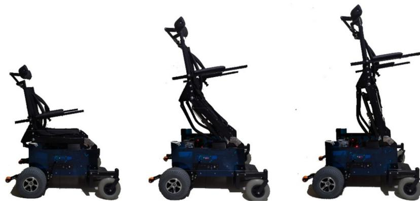
Figure 7. Standing wheelchair at different positions.
