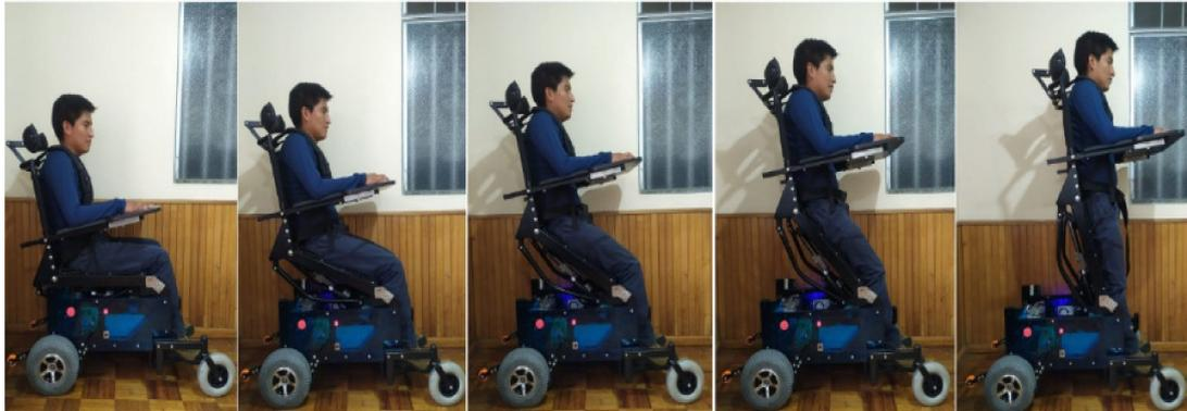
**Figure 11.** Autonomous movement of the standing human–wheelchair system.
