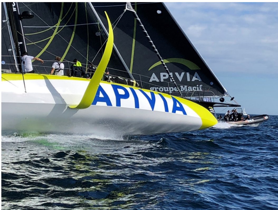
Figure 1. Photograph of IMOCA class APIVIA racing boat, the hydrofoils are manufactured using AFP technology: Photo C. Baley.
