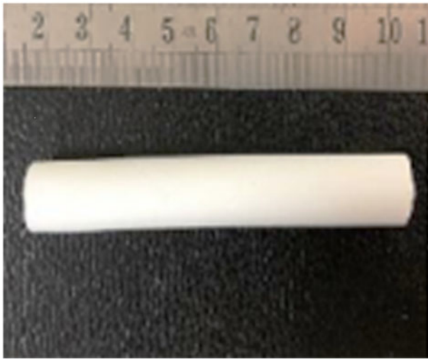
Figure 1. Porous bioceramic rod (diameter: 10 mm, length: 80 mm, macro-pore: 500–600 \mu\text{m} , interconnection: 120 \mu\text{m} ). Reprinted from Ref. [31] with permission
