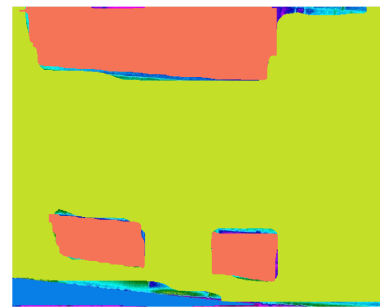
(b) Example of model inference on the Wahpeton State Building. The metrics achieved were 0.76 @ mAP 0.25, 0.64 @ mAP 0.5, and 0.60 @ mAP 0.75 with a mIoU of 0.65
