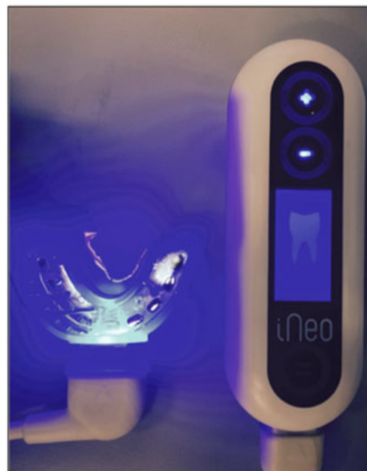
Figure 2. iNéo experimental device allowing the production of 5 mA DCs in the illuminated recipient during the ex vivo antimicrobial procedure of the human dental biofilms.
