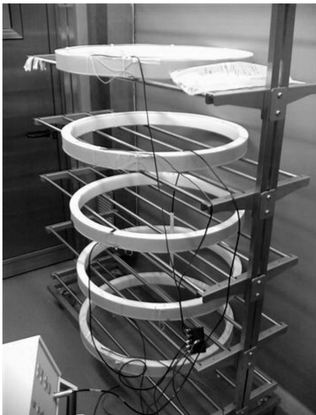
Figure 1 Set of exposure. Each coil has a diameter of 75 cm and the distance between cages is 37 cm.
