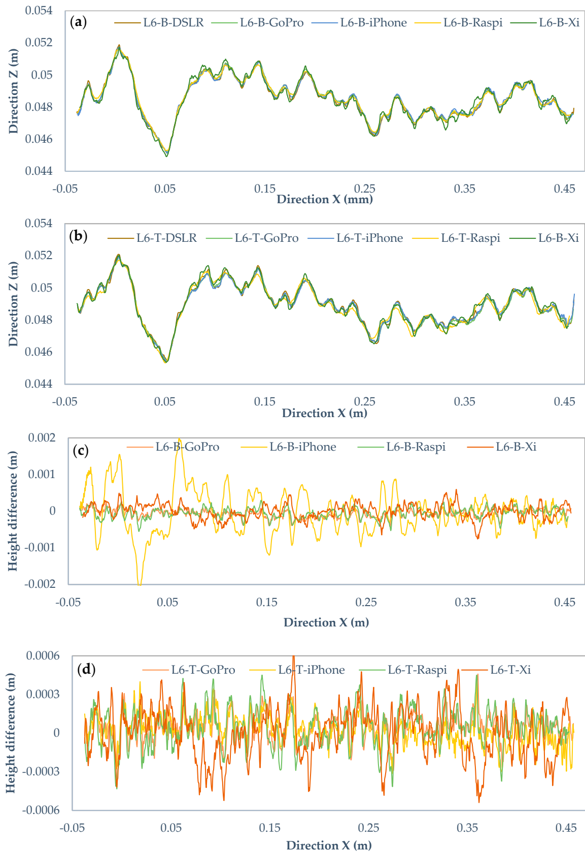
Figure 15. Comparison of the Canon EOS 5DS R DSLR and camera profiles with 0.5 mm rasterization grid interval. (a) Original profiles of bottom surface, (b) top surface, (c) height differences of bottom profiles, and (d) top profiles.
