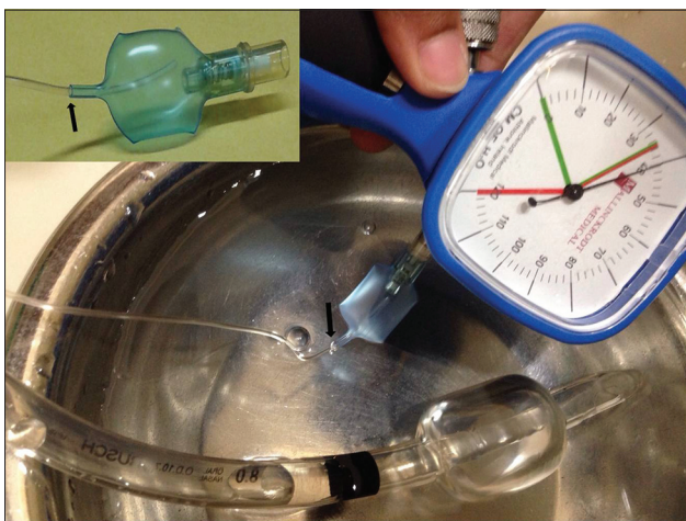
Figure 1: Arrow showing air bubbles in water at higher cuff pressure; inset showing pilot inflation line entering the pilot cuff with the arrow showing the probable leak site
