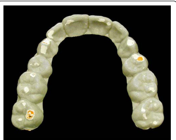
Figure 1 The BBMD, worn by a SB-patient for five consecutive nights, showing all abraded layers of the plate.
